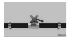
Never use ball valves to regulate flow, but only to intercept fluids to intercept fuids, so to avoid damages to gaskets.
